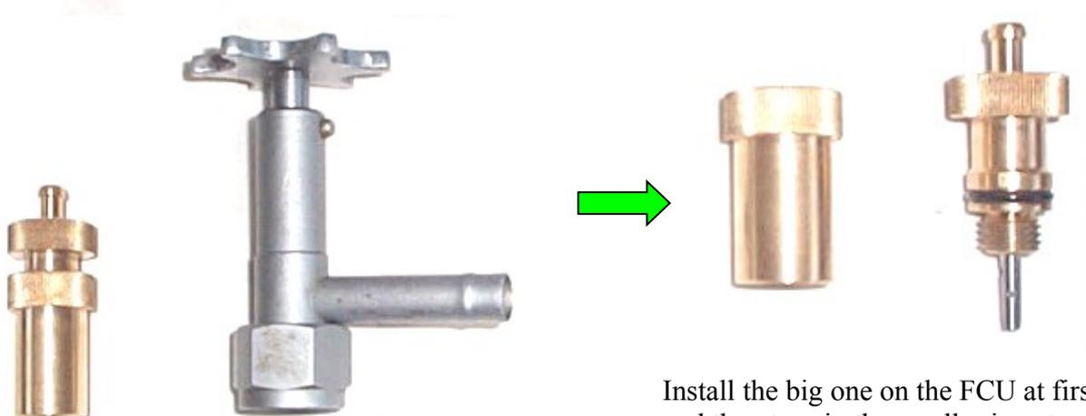
Better handling than the originals, more clearance to the oil lines above the bleeder valve of the FCU
